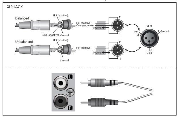
Connect a stereo output source device to the RCA connectors of the INPUT 2. (Unbalanced, OdBV/1Vrms)
